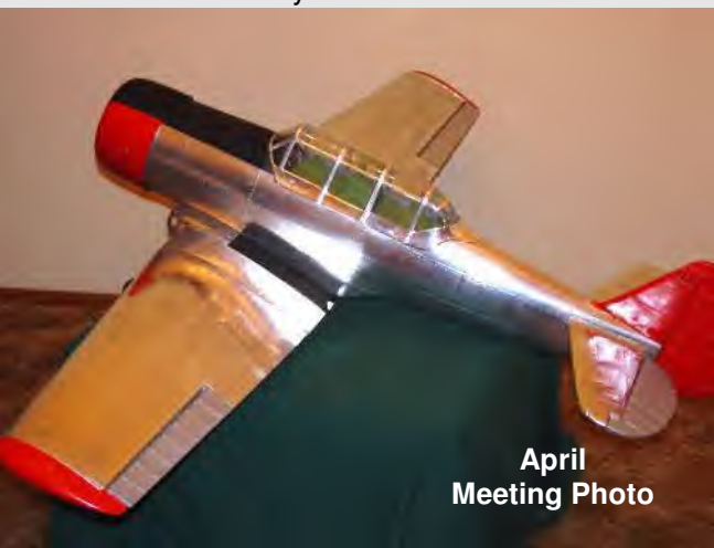
Joe Halamek .015 Aluminum Covered AT-6 Rivets & panels
